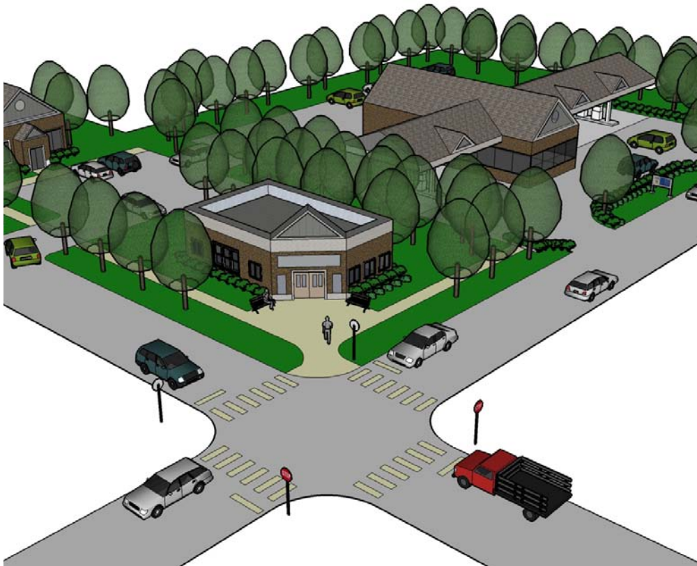
(b) Building on corner lot properly oriented towards both roads
